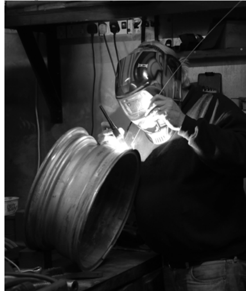
At this stage you look away as Eddie applies filler rod to build the alloy profile back.
