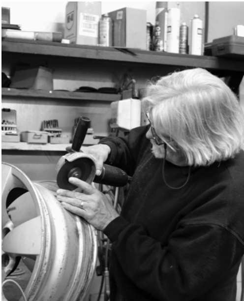
Eddie gets the cracked section removed.
